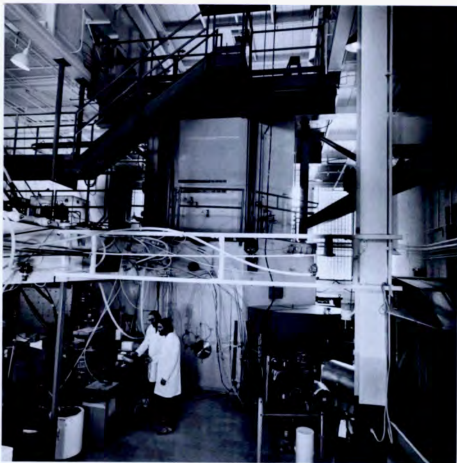
Fig. 7. North face of the Omega West Reactor. The numerous tubes above and behind the two employees are associated with automated neutron-activation analysis facilities.
